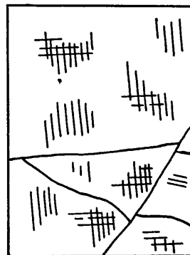
Fig. 1. Traces of habit plane on a \{110\} plane of a transformed single crystal of cubic zirconium, obtained with Roberson's etching reagent No. 3. Schematic drawing from actual photograph (magnification 50\times ).
